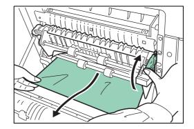
4 If there is jammed paper in the output section, remove it.
